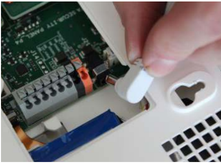
Plug in the power connector
