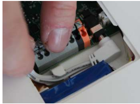
Route the wire behind the retainer clip
